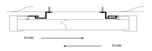
5. Screw the screws (E) into the holes found on both sides of the product and tighten.
